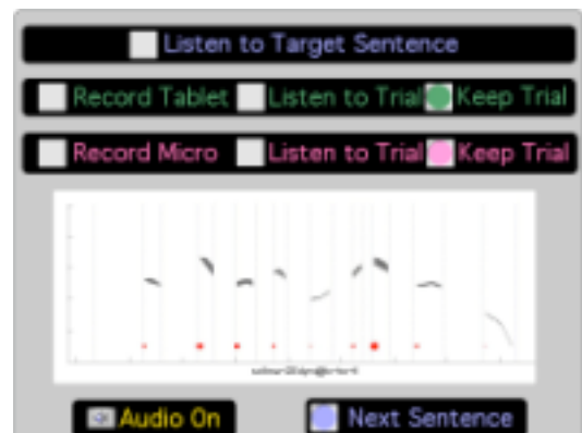
Figure 3: interface used for the handwriting imitation of prosody. Buttons allow to listen to the original sentence, record its own speech or the graphic tablet, listen to a recorded performance and save it. The current sentence’s F0 is displayed.
