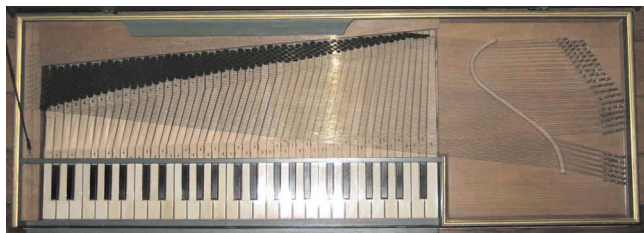
FIG. 1. (Color online) The Bal-Sidey clavichord studied in this article (51 keys, C1-D5, unfretted), dimensions 110 \times 36.5 \times 11 cm.
